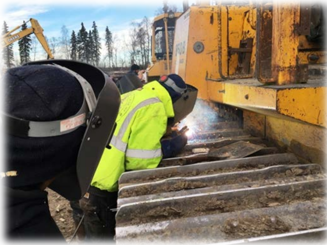
Dakota welding ice cleats on the dozer track
