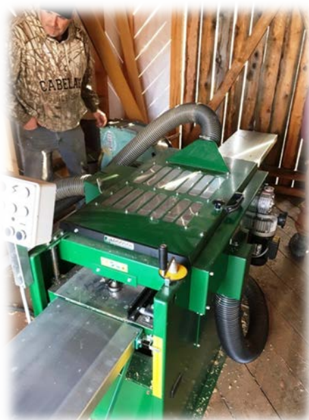
Value-added products: planer –molder that can make tongue & groove and many other finished wood products
