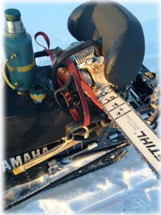
Break time for crew & equipment: Chain saw with marked bar cuts hundreds of test holes in the ice. We are looking for 24" minimum for our plowing equipment
