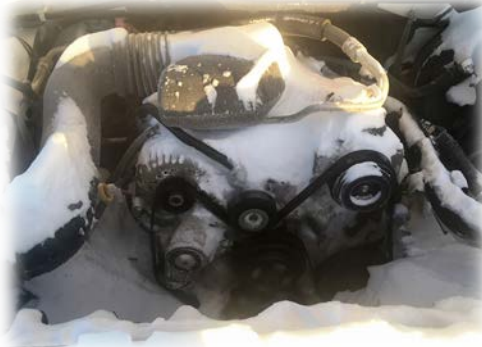
Knowing When to Turn Back: road to Kasigluk in 1-19 storm Engine compartment full of snow – losing electrical power
