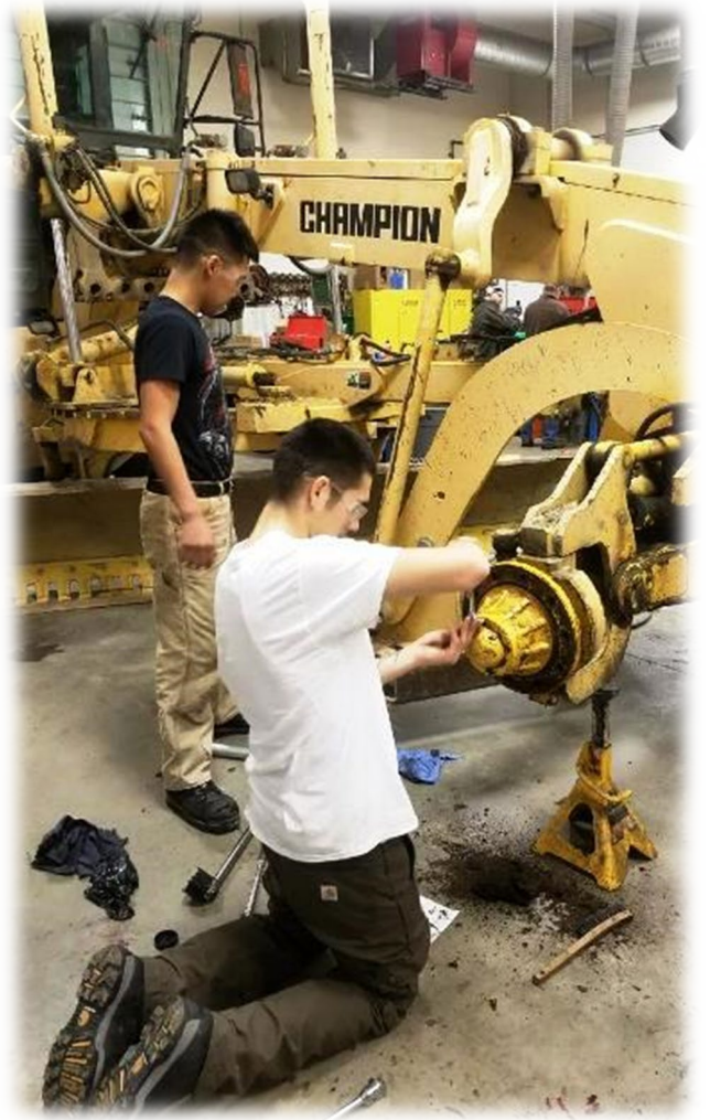
Joey Davis disassembles the front end of a road grader
